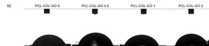
Fig. 3. a) Comparison of wettability tests carried out in water and acquired over time of fibers tablets (mean values \pm s.d.; n=3); b) images acquired during the contact angle measurement after 1500ms from the drop of water falling on the fibers; ANOVA 1 way, Test Scheffé
