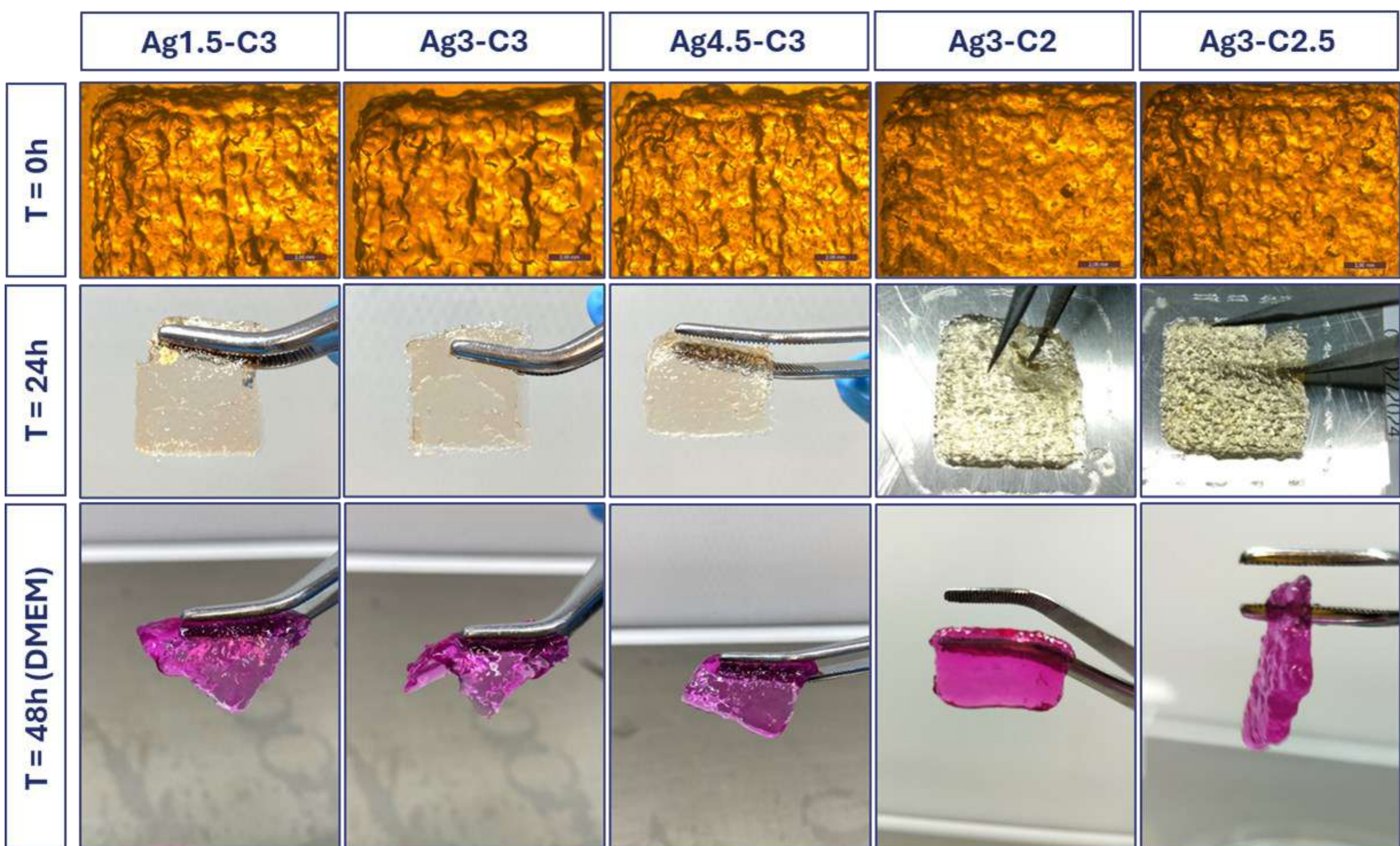
Figure 1. Printed structures: handling and swelling in DMEM
